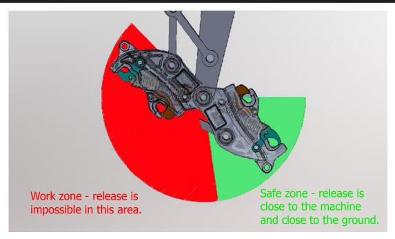
The built-in Smart Valve prevents release until the coupler is in the release zone.
